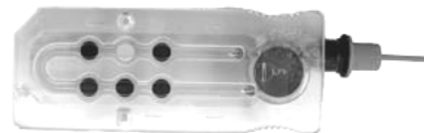
Figure F-4: IDEXX VetStat cassette with syringe adapter attached, Becton Dickinson 1-mL syringe
